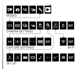
\* Not shown on Hero3+ cameras \*\* Playback only appears if connected to TV or LCD Touch BacPac.
